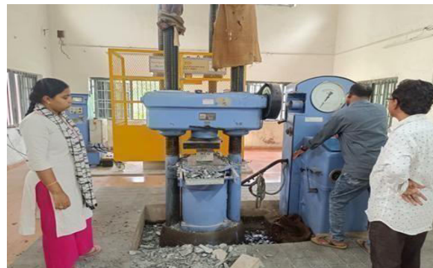
Fig 2: Compression test for cube specimens
