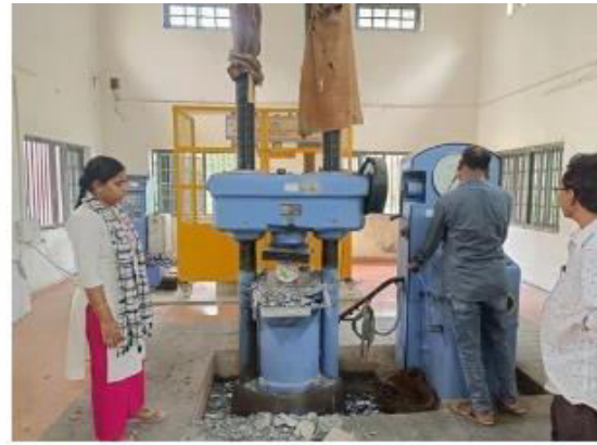
Fig 4: Split Tensile Strength test for cylinder specimens
